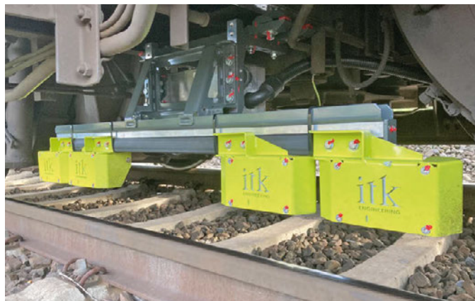
Magnetic Railway Onboard Sensor (Maros) Magnetic Railway Onboard Sensor (Maros)
